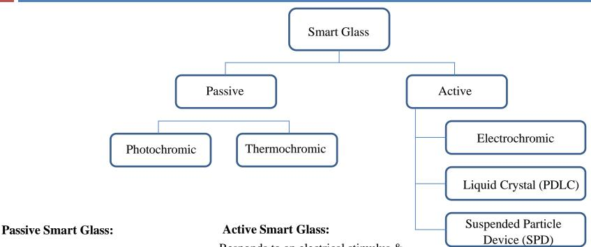
Responds to non-electrical stimuli (heat, UV). Cannot be manually controlled Responds to an electrical stimulus & and is controllable manually or automatically
